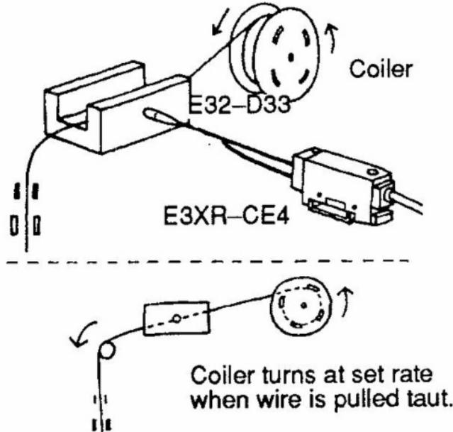
Fiber Optic Photoelectric Switch
